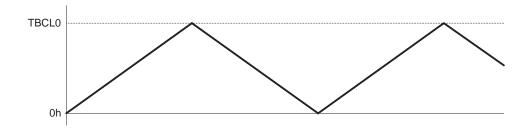
The count direction is latched. This allows the timer to be stopped and then restarted in the same direction it was counting before it was stopped. If this is not desired, the TBCLR bit must be used to clear the direction. The TBCLR bit also clears the TBR value and the TBCLK divider.
